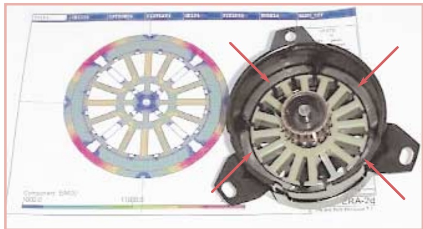
A disassembled ECF motor has four new injection-molded Neo arcs installed (arrows), and the armature winding removed in preparation for rewinding.
